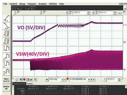
1. The output of a forward converter during startup mode, with a load applied at 10 V, shows the system power-cycling and the output overshooting by about 10%.
