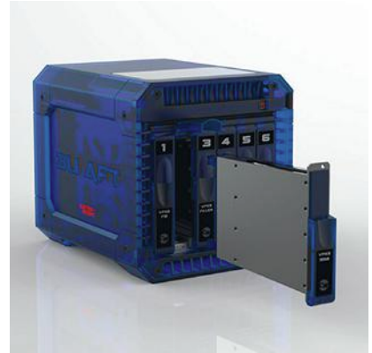
3. A VITA 48.8 frame no longer has to act as a conduction-cooling system. Thus, it can be made out of lighter materials such as this Curtiss-Wright 3D-printed plastic case.
