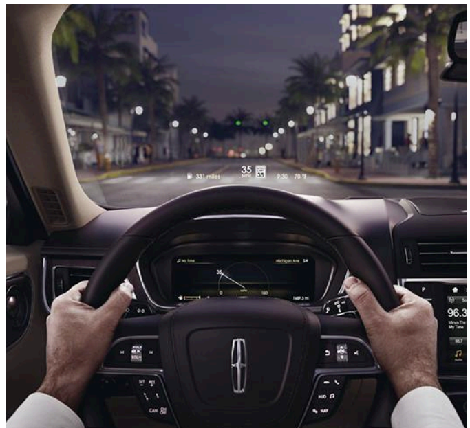
1. Shown is a head-up display feature in the 2017 Lincoln Continental. (Courtesy of Texas Instruments)
